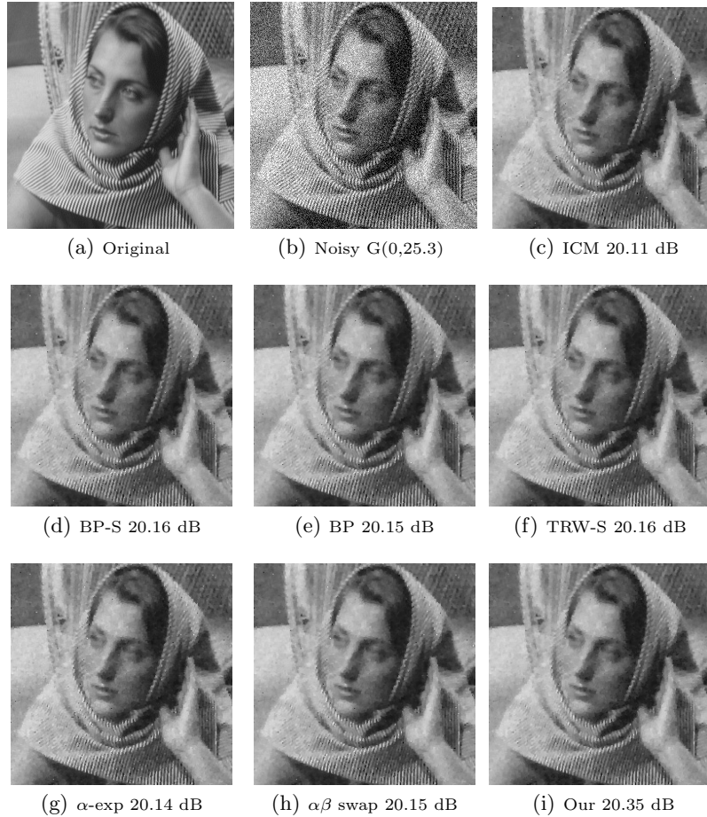
Fig. 3. The image restoration results for truncated \ell_1 - \ell_2 prior with threshold T = 50 , \ell_2 data fidelity term, and \lambda = 2
